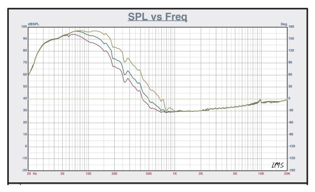
\*Yellow, Green and Red Graphs indicates FREQ knob adjustment for 150Hz, 120Hz and 80Hz respectively.
